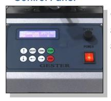
COUNTER: set and record the test times.
