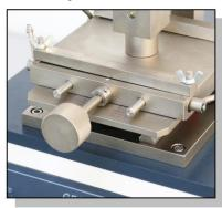
To adjust the distance between the front fixture and rear fixture
